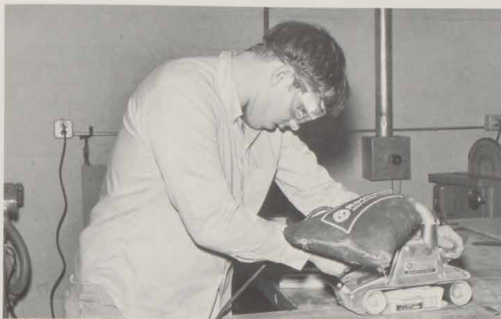
Sanding a piece of lumber is just one step which Danny Brim must execute in order to complete his senior project in woodworking.
